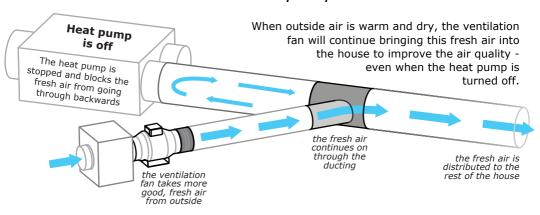
The ducting after the fan can be split into several branches in order to connect to all the required heat pump ducting branches. The splitters are connected after the fan and acoustic ducting - the backdraft shutter can be placed directly on the fan outlet side.
