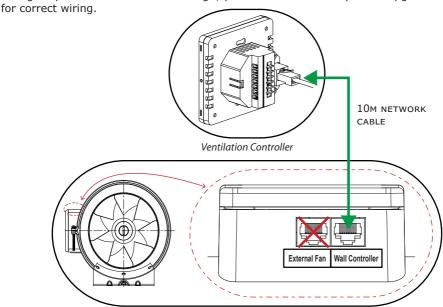
EVOAQ Heat Pump Injection Ventilation Fan
